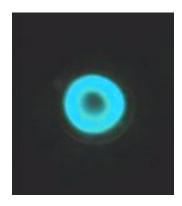
This variation is not perceived by the outside observer, as he cannot see what happens inside the plasma column. However, in this picture we clearly see that the current flow is moved to the external layers of the electrode. Therefore, we have a hollow plasma column. As the effective area of the plasma column decreases, current density increases. Therefore, the MOR causes a shift in the spectral output.
