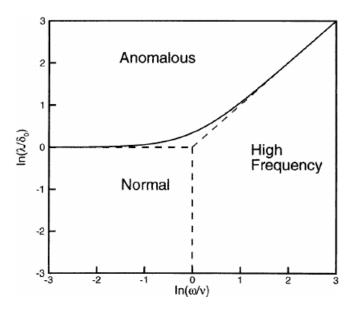
The anomalous skin effect also shows us that the diathermy machine practically only serves the required current, as its RF component is damped. The only effective component acting on current density becomes the MOR, which must compensate to counteract the anomalous skin effect at full regimen.
